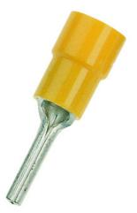
Crimp lug, Pin shape acc. to DIN 46231, Length: 25.5 mm, Max. wire cross-section: 6 mm<sup>2</sup>, Colour: Yellow
