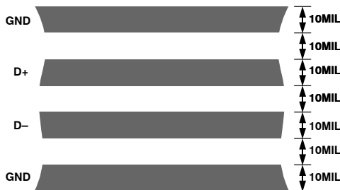
Figure 34. Arrangement of Signal Tracks
