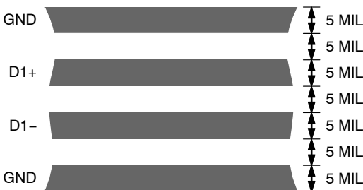
Figure 17. Arrangement of Signal Tracks
