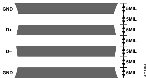
Figure 25. Arrangement of Signal Tracks
