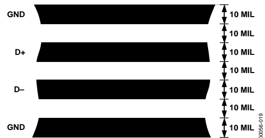
Figure 19. Arrangement of Signal Tracks
