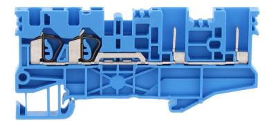
Feed-through terminal, Tension-spring connection, Mounting type: Mounting rail TS 35/7.5, Rated cross-section: 2.5 mm<sup>2</sup>, Width: 5.1 mm, Colour: Blue
