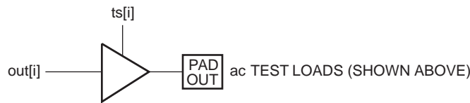
Figure 57. ac Test Loads
