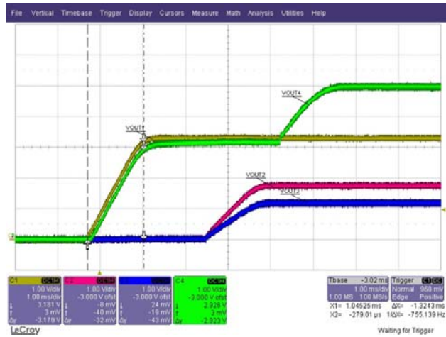
Figure 40. Soft Start Timing
