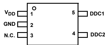
ISL54103 (5 LD SOT-23) TOP VIEW
