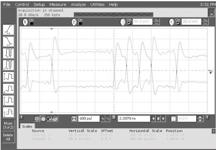
Data Waveforms, 2.5Gbps (left) & 5.0Gbps (right)
