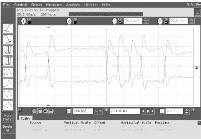
Data Waveforms, 3.0Gbps (left) & 6.0Gbps (right)
