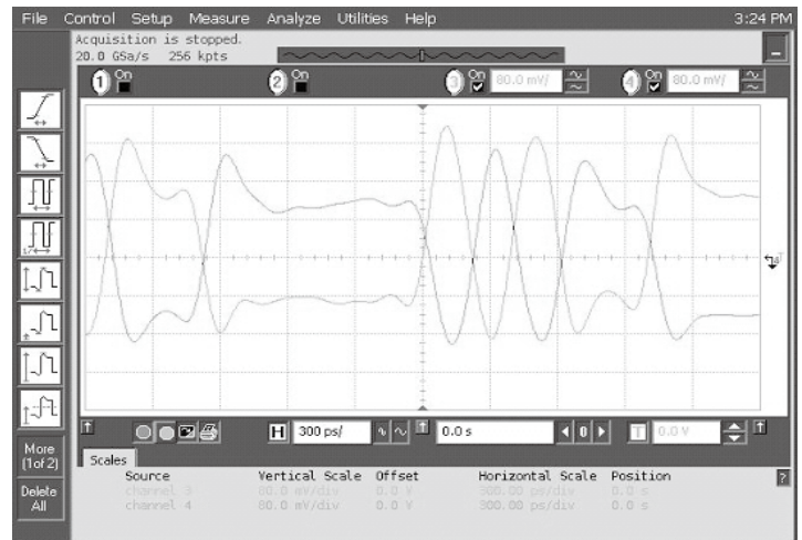
Data Waveforms, 3.0Gbps (left) & 6.0Gbps (right)
