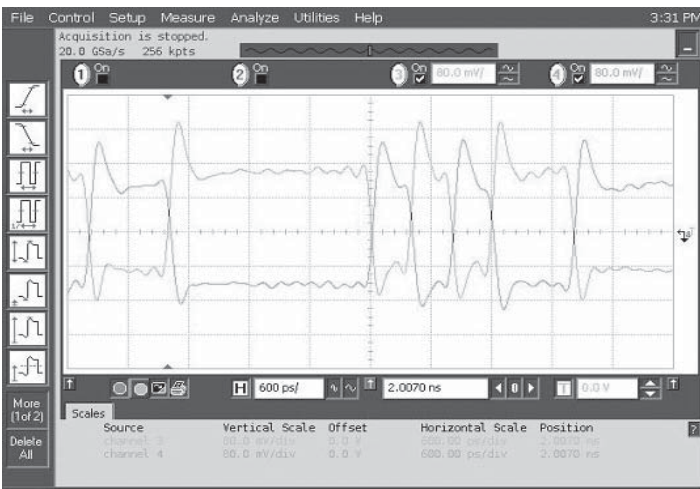
Data Waveforms, 2.5Gbps (left) & 5.0Gbps (right)
