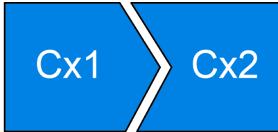
Figure 6.1 : Self Capacitance Swipe Switch Sample Electrodes.
