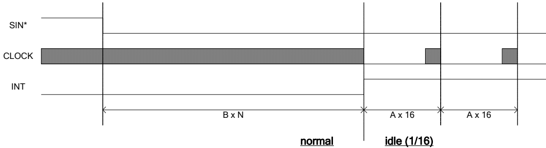
INT pin condition 1 (normal → idle)
