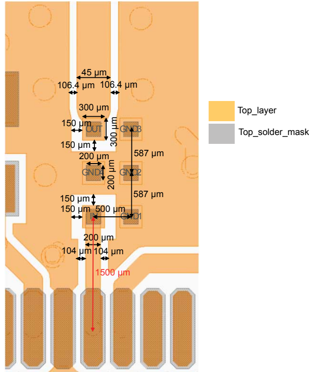
Figure 13. PCB land pattern recommendations
