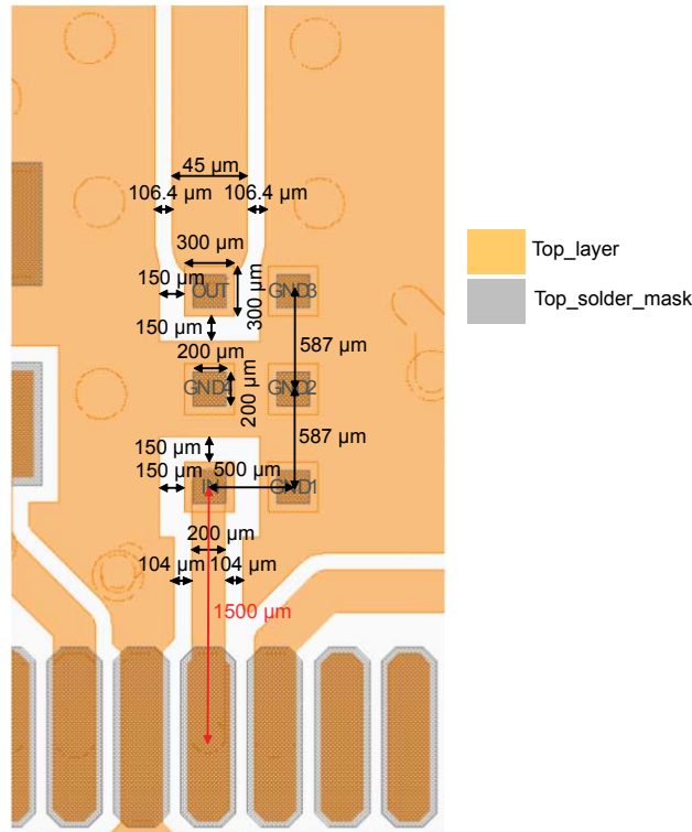
Figure 9. PCB land pattern recommendations
