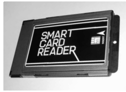
Contact type reader/writer RW-4020 (LR550R03)
