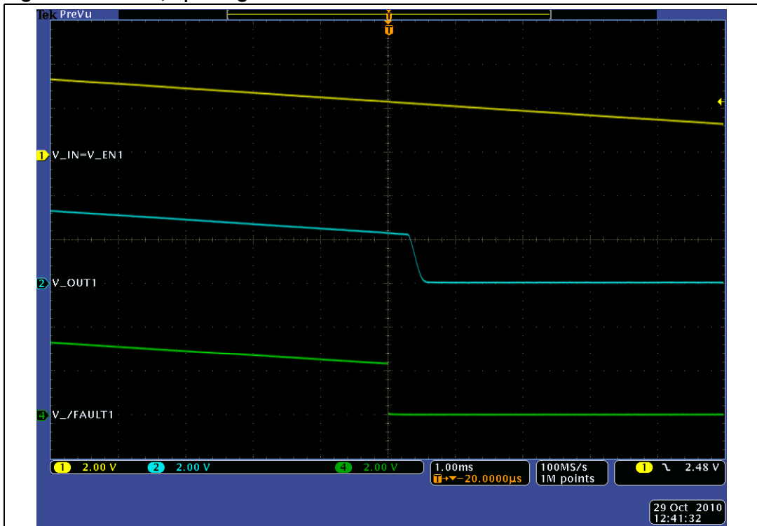
Figure 16. UVLO, V_I falling
