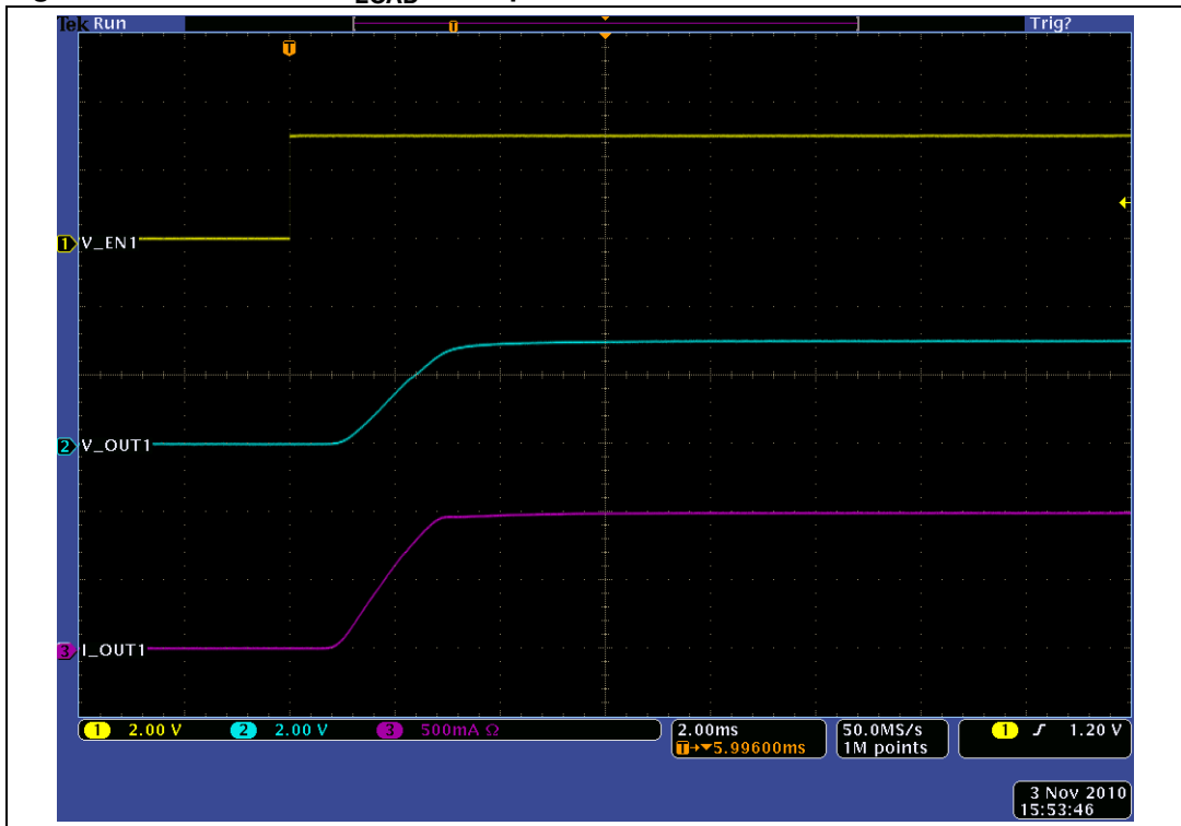
Figure 25. Turn-on for C_{LOAD} = 470 \mu F
