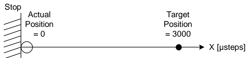
Figure 23: Positioning Example: Situation after reference search
