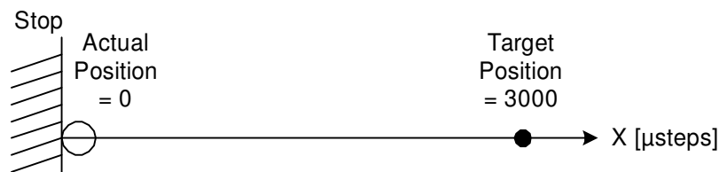
Figure 23: Positioning Example: Situation after reference search
