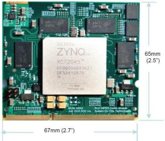
Fig.5 The SOC SoM-X-Z7045 Module
