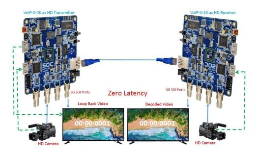
Fig. 11 Setup for the SOC HD video encoder-decoder evaluation and latency evaluation using the VoIP-X-4K kit
