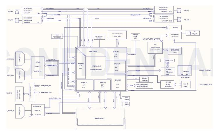
Fig. 12 Block diagram of VoIP-X-4K board
