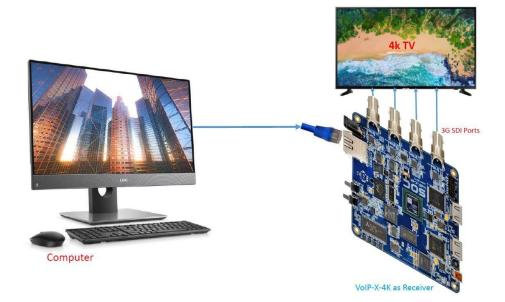
Fig. 9 Setup for the SOC 4K video decoder evaluation using the VoIP-X-4K kit
