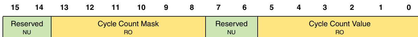
Figure 3-129. CCFnR, CC Part Buffer of a Double Transmit Message Buffer Filter Registers
