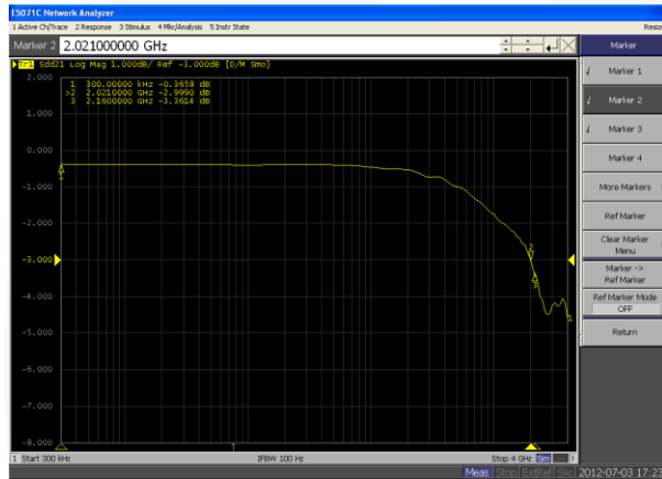
Figure 17. MHL Path SDD21 Insertion Loss Curve
