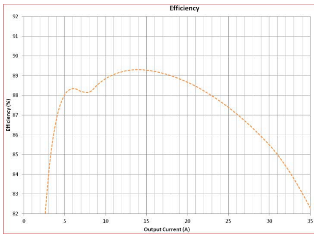
Figure 5. Efficiency – 19 V Input, 1.2 V Output, 500 kHz
