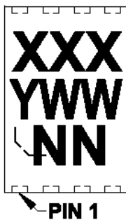
8-Lead TDFN (2x3x0.75 mm)
