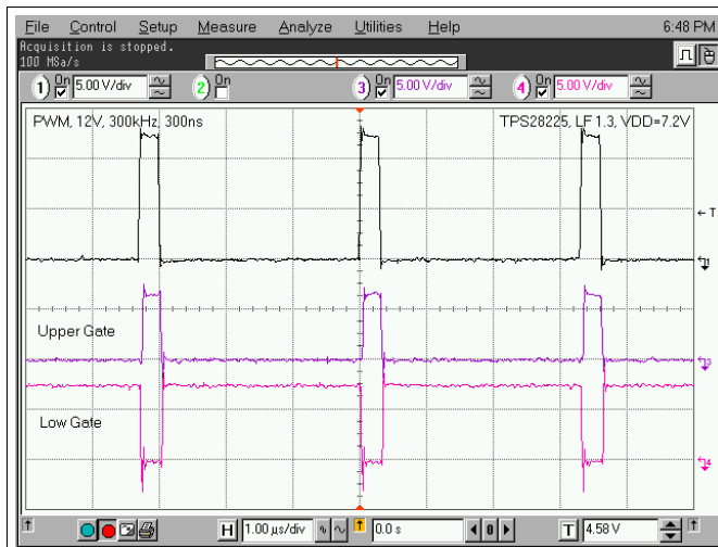
Figure 23. 12-V PWM Pulse at V_{DD} = 7.2\text{ V}
