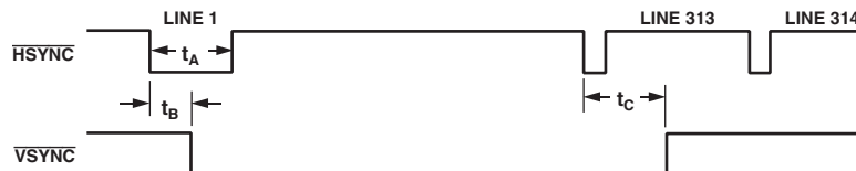
Figure 21. Timing Register 1 in PAL Mode
