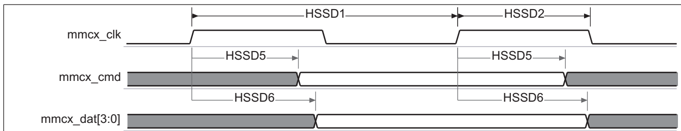
Figure 6-65. MMC/SD/SDIO – High-Speed SD Mode – Data/Command Receive
