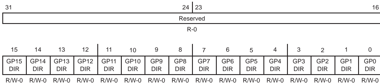
Figure 7. GPIO Direction Register (GPDIR) [Hex Address: 01B0 0004]
