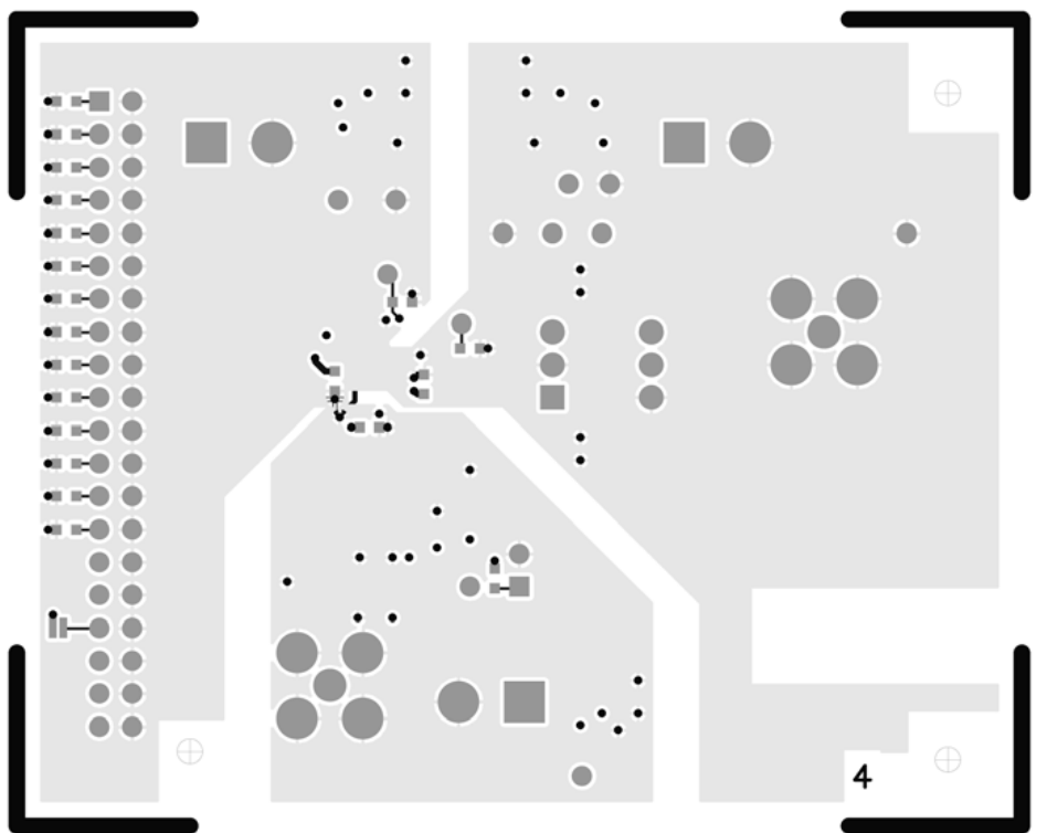
Figure 36. Evaluation Board Layout—Secondary Side
