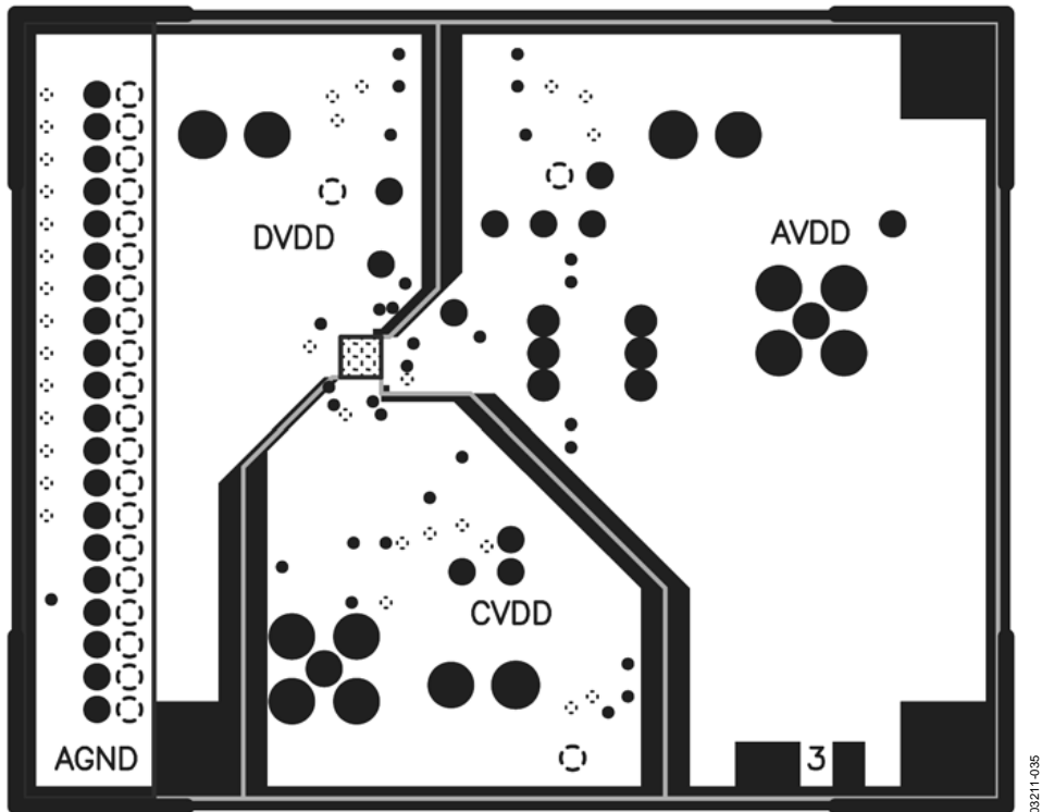
Figure 38. Evaluation Board Layout—Power Plane
