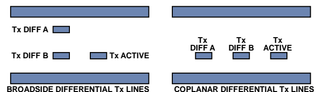
Figure 66. Broadside vs. Coplanar Differential Stripline Routing Techniques
