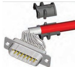
Attach the strain relief around the cable
