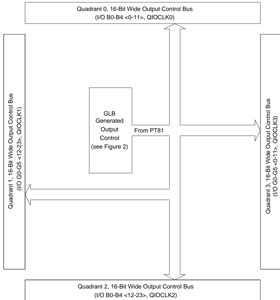
Figure 5. Output Control Bus and Quadrant Organization
