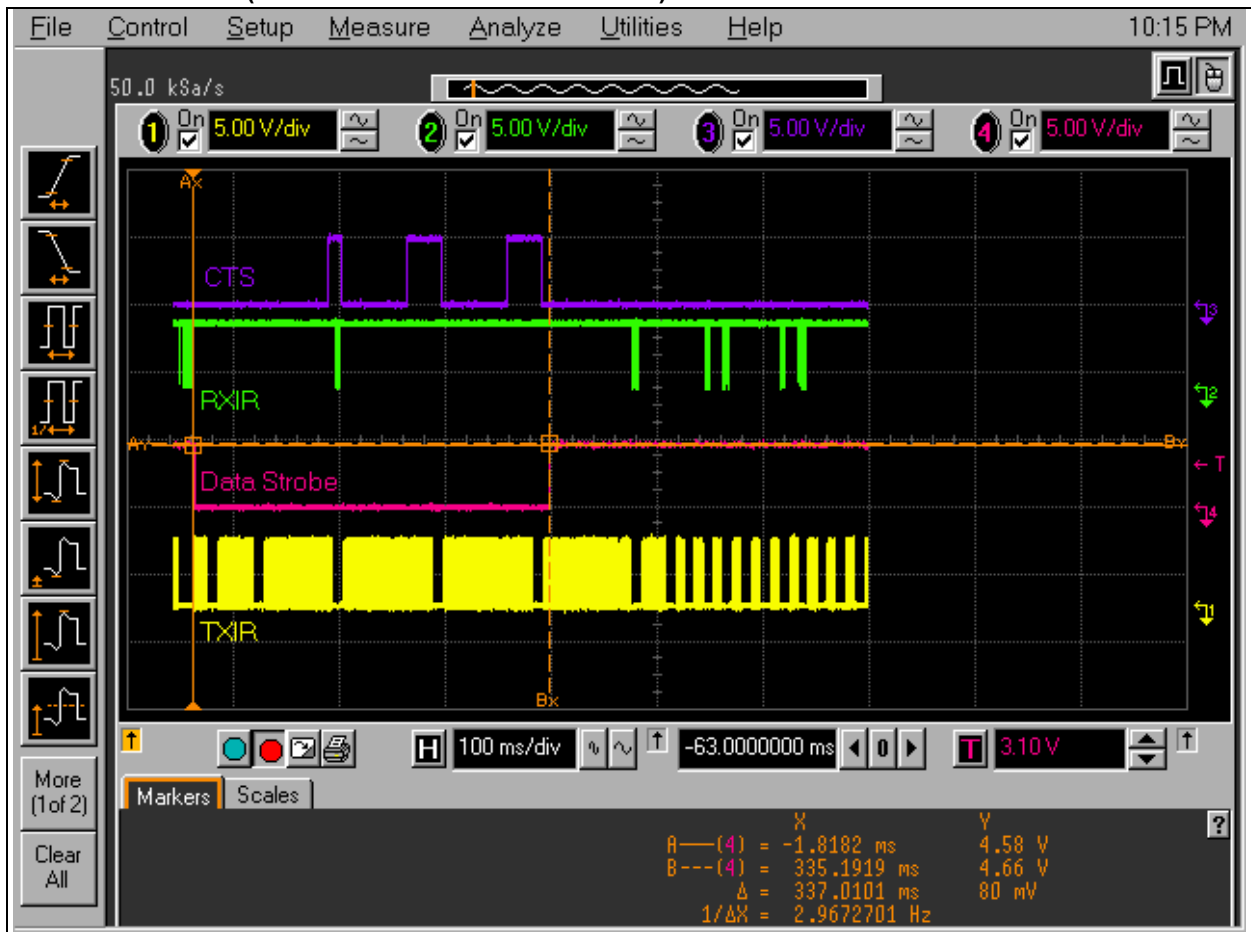
FIGURE 2-12: HOST CONTROLLER TRANSMISSION (S → P) OF A 250 BYTE PACKET (TO PIC IrDA STANDARD STACK)
