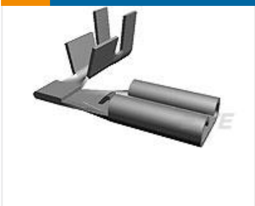
TE Part #62336-1 110 FASTON FLAG REC 22-18 AWG TPBR
