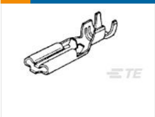
TE Part #174777-1 PL 110 REC 20-16 AWG 0.25 X 10.4 PTBR
