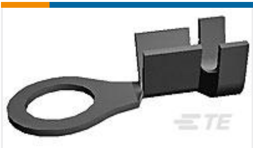
TE Part #61352-1 RING .197 (5.0 MM) 10-6 AWG TPBR
