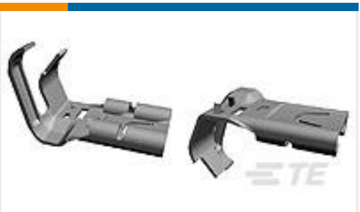
TE Part #63604-1 250 FASTON FLAG REC 18-12 AWG NPST
