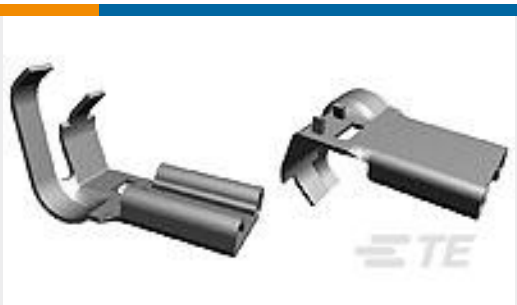
TE Part #42742-2 250 FASTON FLAG REC 18-12 AWG TPBR
