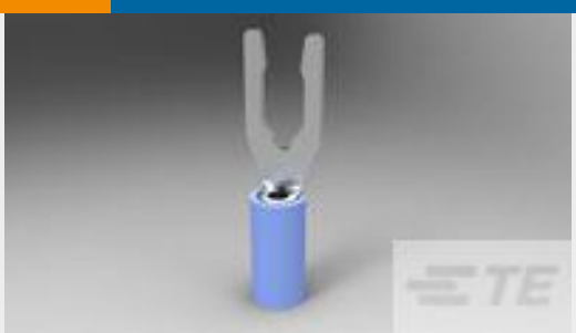
TE Part #52421-3 TERMINAL,PIDG SPR SPD 16-14 8
