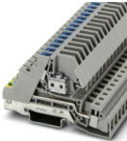
Installation level terminal block, Screw connection, Cross section: 0.2 mm 2 - 10 mm 2 , AWG: 24 - 8, Width: 8.2 mm, Color: gray, Mounting type: NS 35/7,5, NS 35/15
