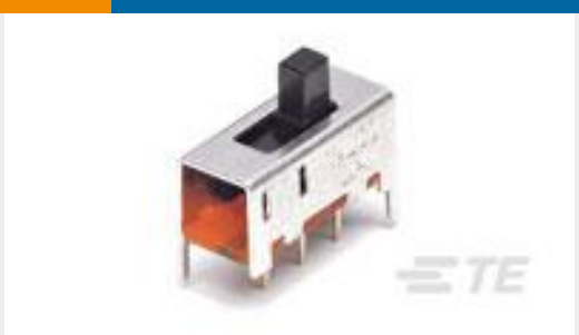
TE Part #1825263-1 MSS225004=DPDT SL SW VERT AG
