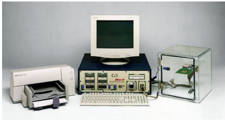
Figure 3-10: \theta_{JA} Measurement Setup
