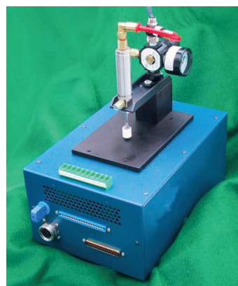
Figure 3-9: \theta_{JC} Measurement Setup
