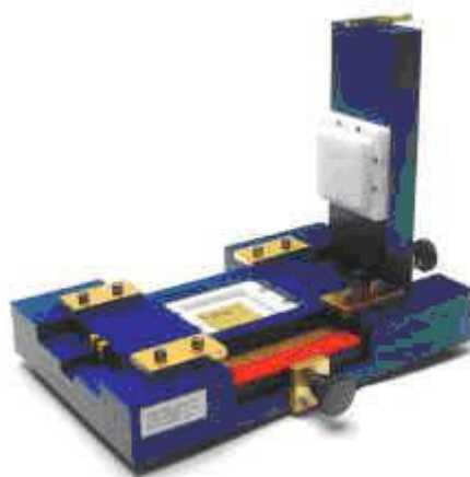
Figure 4-1: Altair BGA Fixture Used for TDR Measurement
