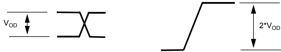
Figure 19 - Differential Output Voltage Parameter
