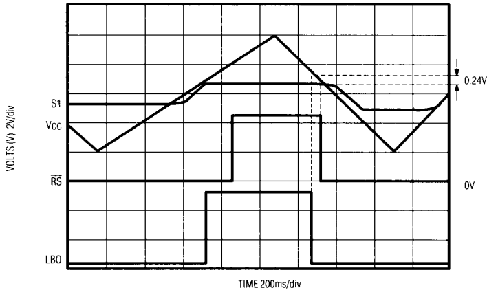
BACKUP-BATTERY SWITCHING AND WARNING FLAGS
