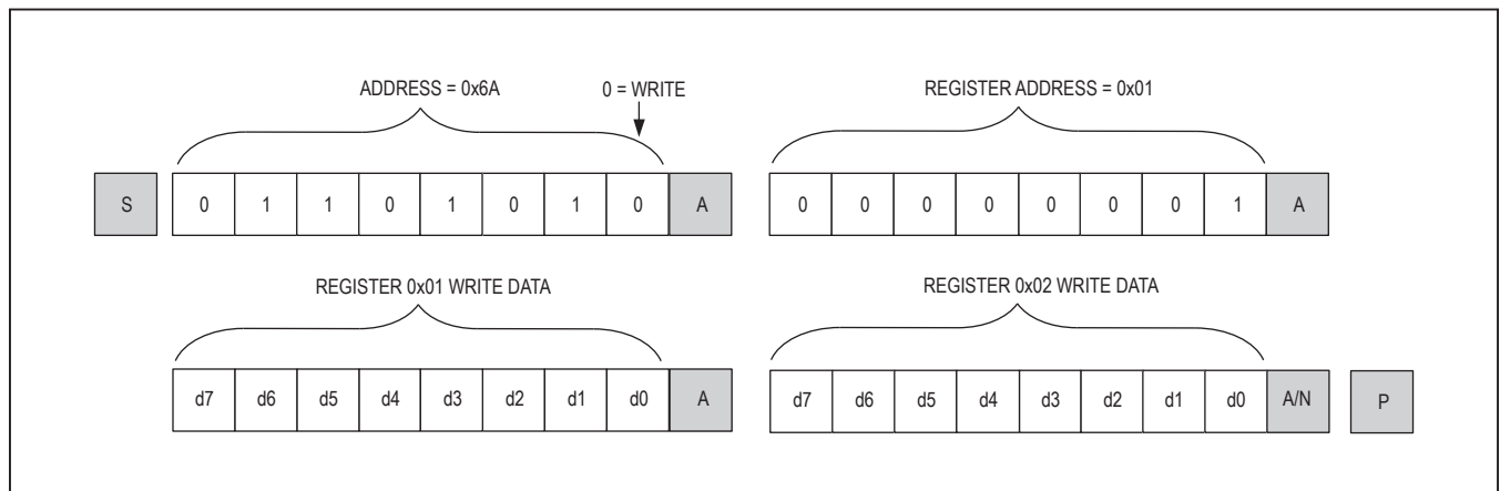
Figure 9. Format for Writing to Multiple Registers
