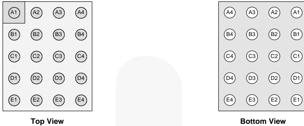
Figure 4. WLCSP-20 Pin Assignments
