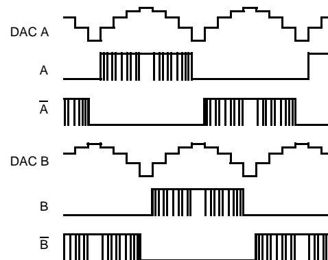
Figure 11: Stepper Motor Waveform - LM9832 Signals
