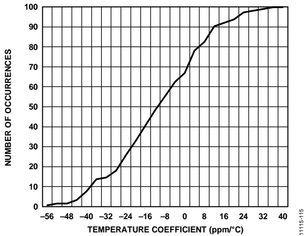
Figure 15. Cumulative Histogram of the Current Channel ADC Gain Temperature Coefficient for Temperatures Between 25^{\circ}\text{C} and 85^{\circ}\text{C}
