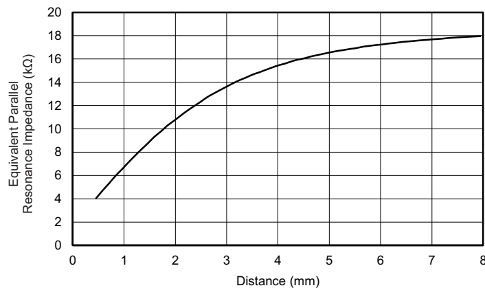
Figure 9. Typical R_p vs Distance With a 14-mm PCB Coil
